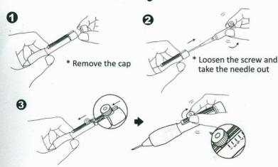
\* Insert the needle into the barrel and tighten the screw once the loop length is determined
